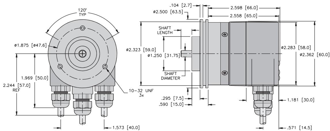
**Sendix absolute, singleturn type 5858 (shaft) / 5878 (blind hollow shaft) PROFIBUS®-DP**
