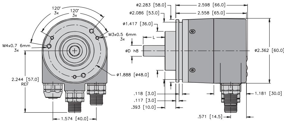
**Sendix absolute, singleturn type 5858 (shaft) / 5878 (blind hollow shaft) PROFIBUS®-DP**
