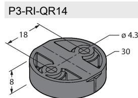
Positioning element for angle sensors RI-QR14, flat design, using shield plate SP1-QR14 is recommended
