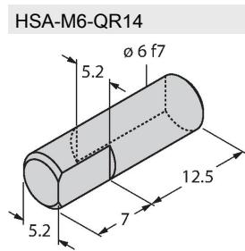
Adapter for RI-QR14 specific positioning elements, hollow on solid shaft, Ø 6 mm
