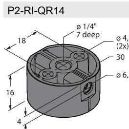
Positioning element for angle sensors RI-QR14, for Ø 6.35 mm shafts
