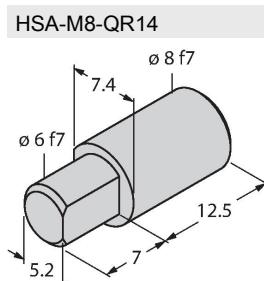
Adapter for RI-QR14 specific positioning elements, hollow on solid shaft, Ø 8 mm
