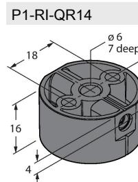
Positioning element for angle sensors RI-QR14, for Ø 6 mm shafts
