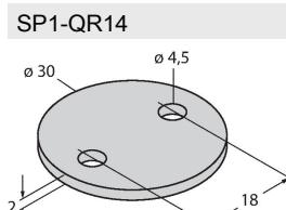
Shield plate Ø 30 mm, aluminium
