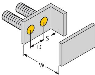
The given minimum distances have been checked against the standard switching distance.
