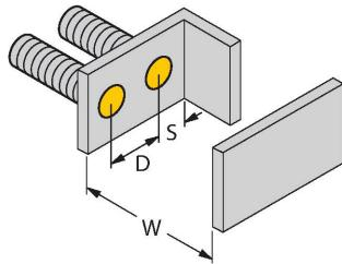
The given minimum distances have been checked against the standard switching distance. Should the sensitivity of the sensors be changed via potentiometer, the data sheet specifications no longer apply.
